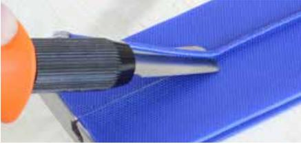
Deburr the protruding bead with the EM01 bead remover. The bevelled blade of the bead remover must be placed at this angle on the belt surface and moved steadily over the seam area.
