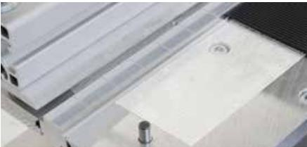
In addition, we recommend that the contact surfaces of the joining table be provided with double-sided adhesive tape flush with the edges in order to simplify the insertion of the flat belt ends, but also to prevent the flat belt ends from slipping during the welding process.
