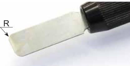
We strongly recommend to grind the corners of the cut surface with a radius before using new blades in order to prevent hook-in or damage to the belt surface during the deburring process.
