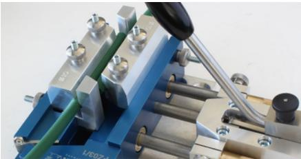
Slide toggle mechanism up to end point.
