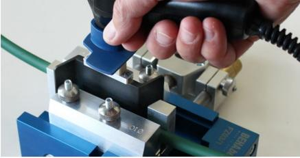
Insert the inspection welding mirror into the gap between the belt ends.
