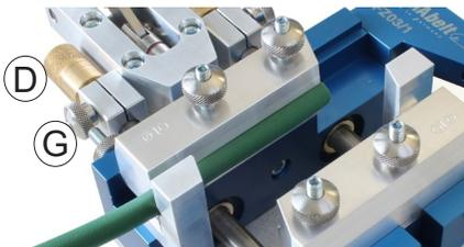
One-sided fastening of belt section in groove of clamping piece.
