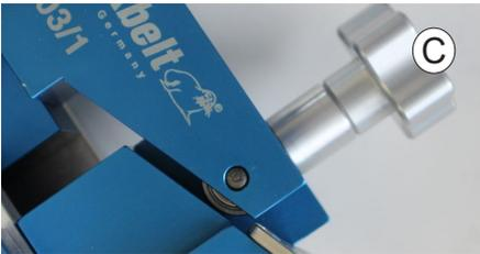
Open toggle mechanism all the way. Open out stop plates for axial contact pressure. Use adjusting knob (C) to adjust ball bearing such that it makes slight contact with the end stop chamfer when the toggle mechanism is closed. Check the position by opening and closing the toggle mechanism.
