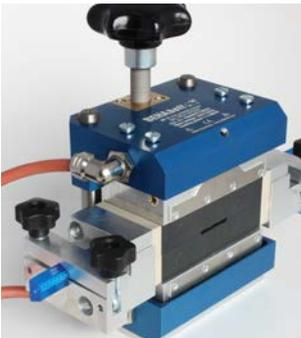
Insert the mould centrally and lengthwise into the press.
