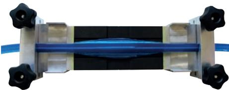
Leave the mould and profile within the closed machine until the temperature is cooled down. The current temperature of the heating plates is shown in the display of PPUs controller.
