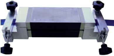
To close the upper part precisely installed on the lower part between the guide webs. During overlap welding the upper part and the lower part initially not touch. The material has yet to be displaced during the welding process or during the holding time.
