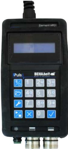
Connect PPuls Controller with the power line and switch on the controller. Selection of welding parameters through direct entry or selection of stored recipes.
